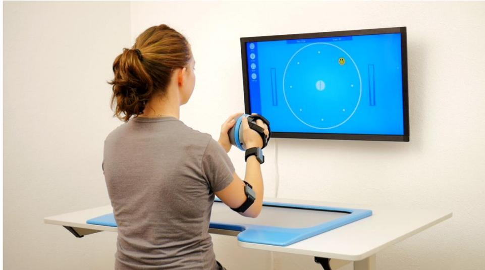
The physical part of the system is divided into three main parts. In the first part, the handle is held by the patient in the affected arm. The handle housing is ergonomically designed and coated with rubber, allowing for reliable and comfortable grip. The three-axis force sensor with a measuring range of  $\pm 100$  N and a resolution of 0,1 N in all directions is mounted in the housing. In addition, an inertial sensor that measures orientation is also present in the housing.
